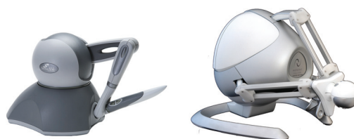
Figure 1: Haptic Devices: the SensAble PHANTOM Omni® is a serial 6DOF input, 3DOF output device ( http://www.sensable.com ), the NOVINT Falcon® is a parallel 3DOF input/output device ( http://www.novint.com ). Photos are courtesy of SensAble and NOVINT.
